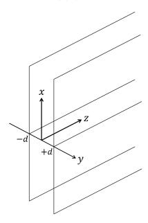
The figure shows a slab of dielectric material which extends to  $\pm \infty$  in the x and z directions but extends only from -d to +d in the y direction. In SI units, the slab has dielectric constant  $\epsilon > \epsilon_0$  and is nonmagnetic. Air ( $\epsilon \approx \epsilon_0$ ) surrounds the slab. We consider an electromagnetic wave propagating in the z direction through the slab. The Maxwell Equations governing this system are given in SI units as
