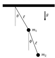
Consider a double pendulum made with masses  $m_1$  and  $m_2$  hanging from a fixed top support by identical massless rods of length  $\ell$ , as shown. A uniform gravitational acceleration g acts on this system.
